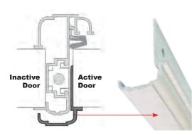
Add an Astragal Security Strip to any outswing double door combination for added security, a clean finished appearance, and eliminate the reveal between the doors.
